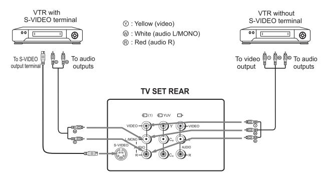
To access the unit connected to these jacks, press TV/AV button until AV1 or SVHS appears on the screen.
